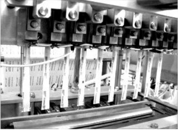
A close-up black and white photograph of the dosing mechanism of a stick packaging machine. It shows ten vertical dosing tracks with hoppers at the top and a collection tray at the bottom.                                             | <p><b><u>Modèle 3</u></b></p> <p>10 pistes de dosage</p> <p>3 g – 5 g – 10 g – 20 g</p> <p>Jusqu'à 300 sticks / min</p> <p>Compatible Papier + PE, PET + PE + film aluminium +PE, OPP+PE, film aluminium +PE</p> <p>Système d'ouverture facile</p> |
