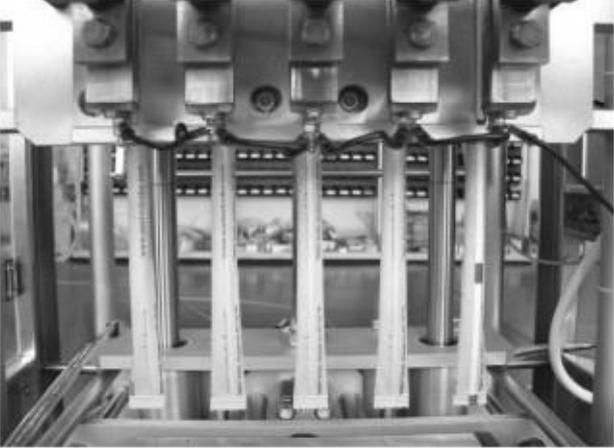
A close-up black and white photograph of the dosing mechanism of a stick packaging machine. It shows five vertical dosing tracks with hoppers at the top and a collection tray at the bottom.                                            | <p><b><u>Modèle 2</u></b></p> <p>5 pistes de dosage</p> <p>5 g- 10 g – 20 g</p> <p>Jusqu'à 190 sticks / min</p> <p>Compatible Papier + PE, PET + PE + film aluminium + PE, OPP + PE, film aluminium +PE</p> <p>Système d'ouverture facile</p>      |
